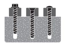
Continue to tighten the anchor until flanged head is firmly seated against fixture. Be sure not to over torque the anchor.
